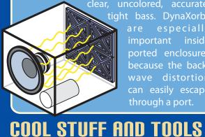
tight bass. DynaXorbs are especially important inside ported enclosures because the backwave distortion can easily escape through a port.
